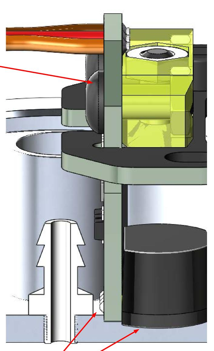
Make sure that the sensor ' face and the backplate are as close as possible by sliding the sensor into the bottom
