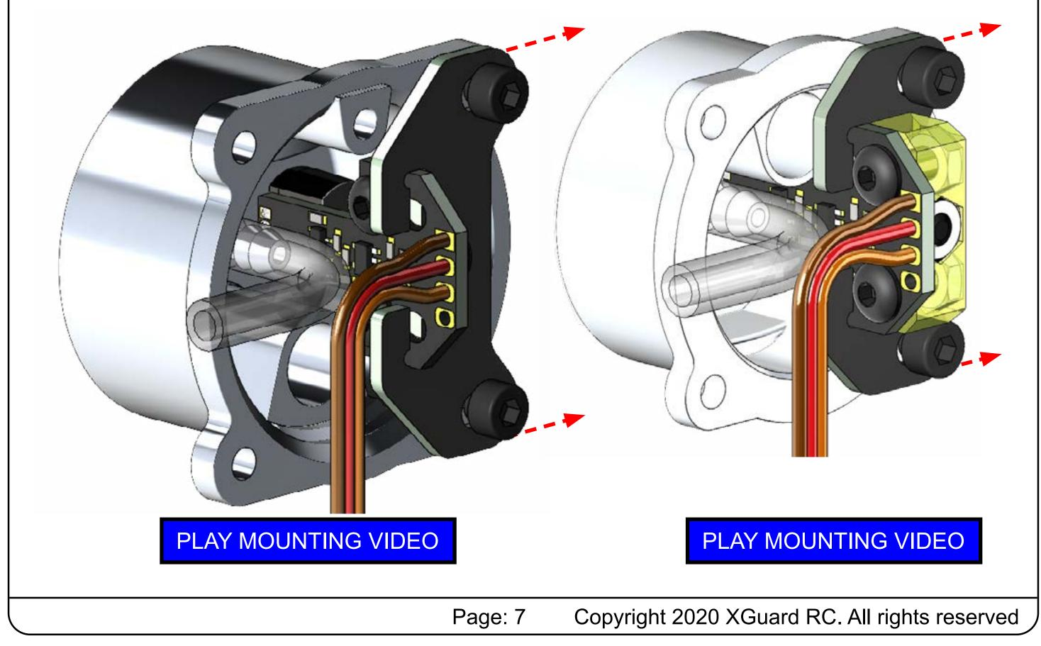
Use these screws to adjust the distance of the sensor face to the backplate bottom
