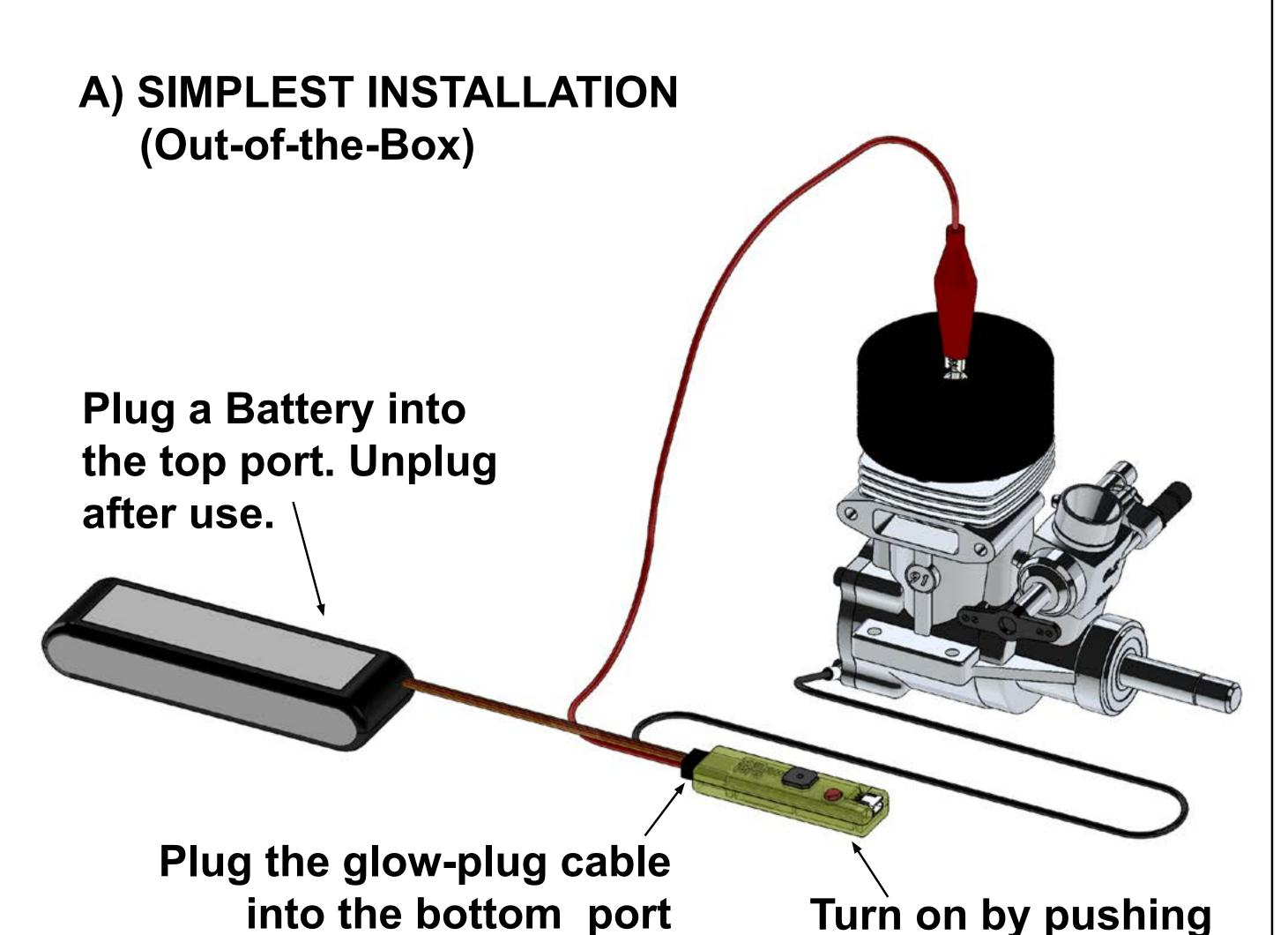
Using this configuration out-of-the-box the unit will use the default Factory settings.
