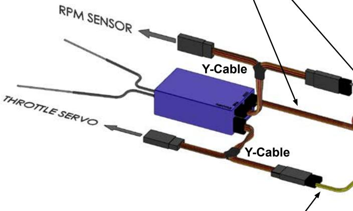
Plug the glow-plug cable into the bottom port and add the throttle pickup wire (SKU: AAVXG0204)
